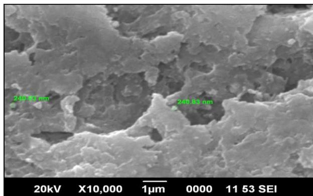
**Figure-5: SEM image of biosynthesized AgNPs from *P.marsupium* bark extract.**
