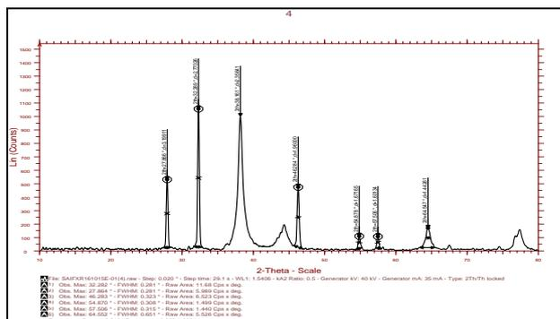
**Figure-4: XRD diffractogram of biosynthesized silver nanoparticles.**
