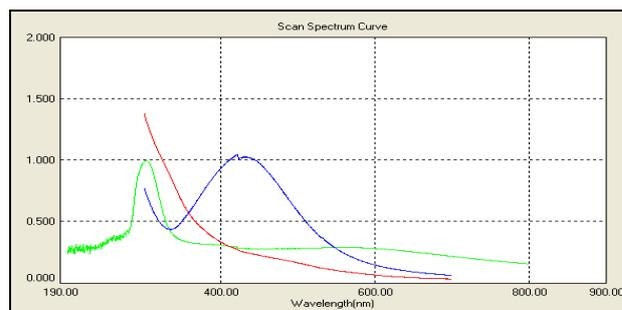
**Figure-2:** UV–Vis absorption peak of *P.marsupium* bark extract (green), AgNO<sub>3</sub> (red) and biosynthesized AgNPs (blue). The absorption spectrum of AgNPs displayed a strong (narrow) peak at 435nm which it is assigned to surface plasmon resonance of the particles.
