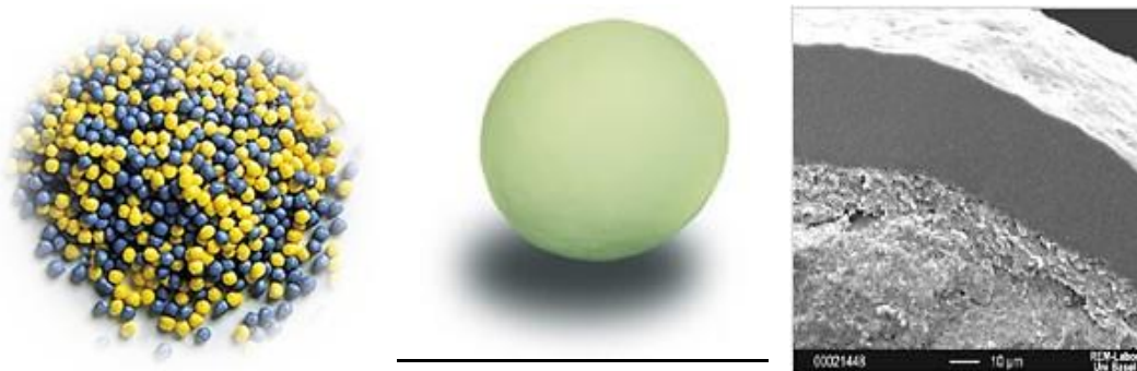
Figure 2 (a) Pellets, (b) Perfect pellet, (c) Coated pellet.
