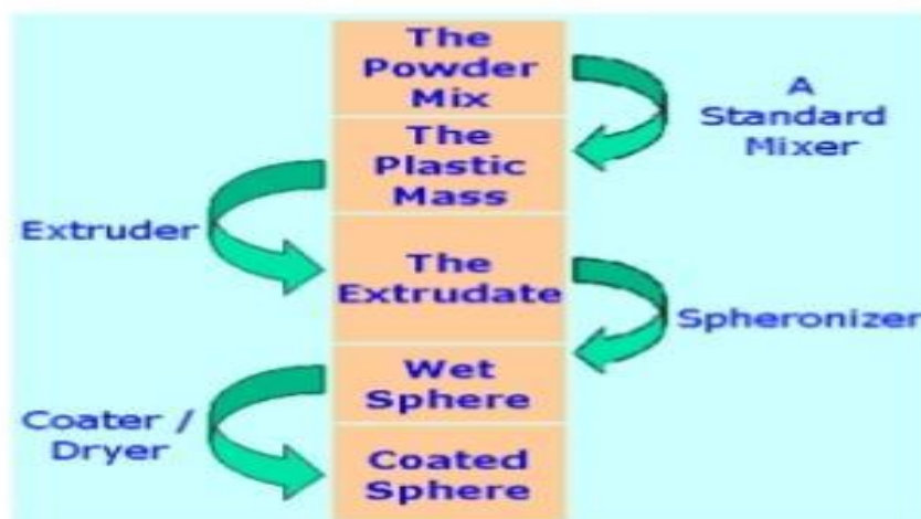
Fig: The extrusion-spheronization process can be broken down.
