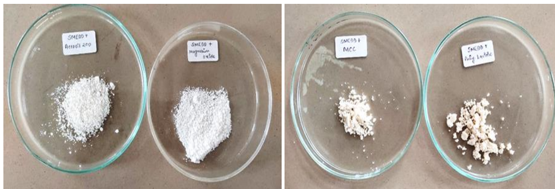
Fig. 1: L-SMEDDS with different adsorbents; colloidal silicon dioxide (OF1SCD), magnesium oxide (OF1SMG), MCC (OF1SMC) and anhydrous lactose (OF1SAL).
