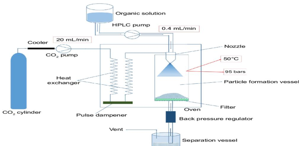
Figure 6: Supercritical Fluid Process.
