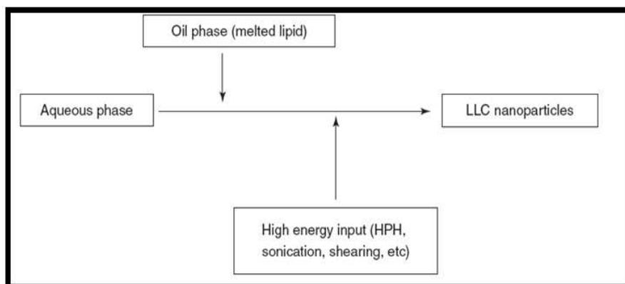
FIG. 2: Top Down approach method.<sup>[17]</sup>
