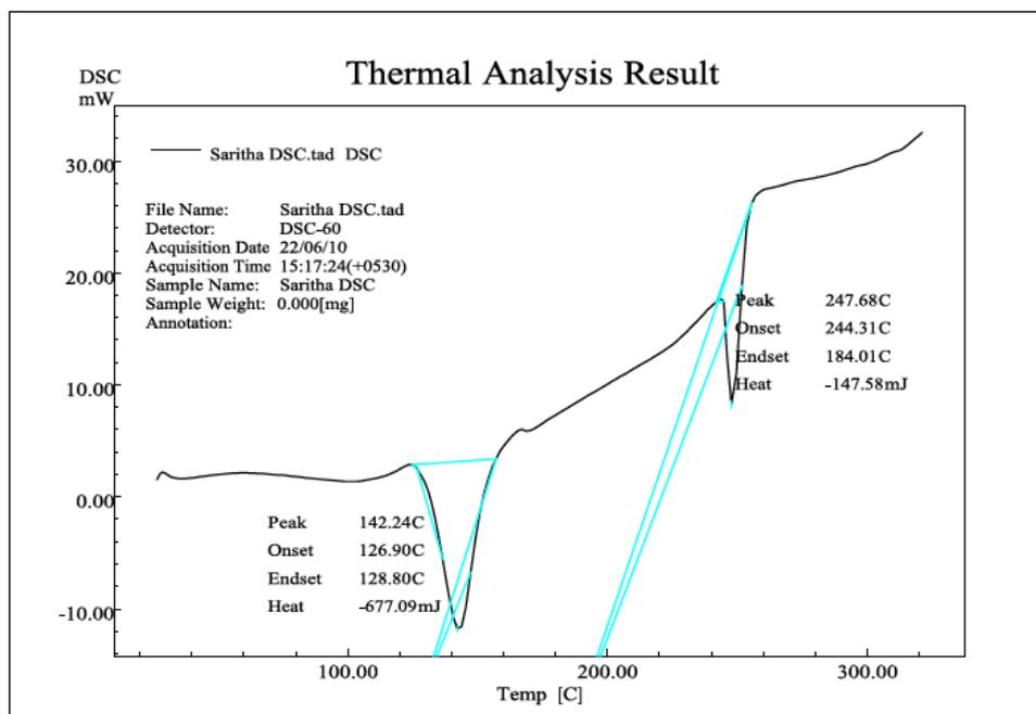
Figure 4: Thermal analysis result.
