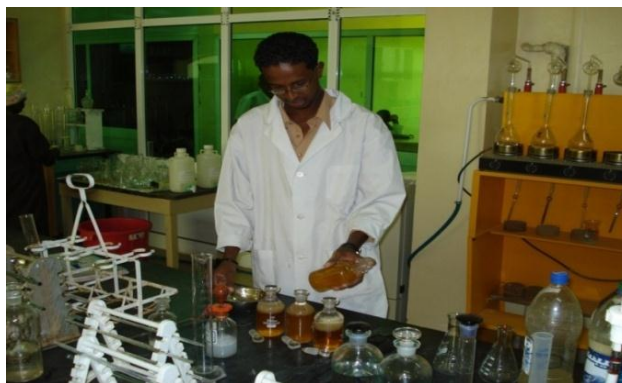
Plate: BOD and DO tests for water samples collected from Kusti town-Sudan.
