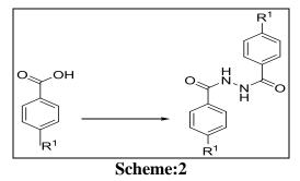
$R^{1}$ =-*CF*<sub>3</sub>,-*F*,-*NO*<sub>2</sub> **Reagents & Reaction Conditions**: SOCl<sub>2</sub> & Hydrazine hydrate
