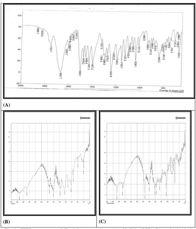
Fig 2. FTIR spectrum of Etodolac pure drug (A), Kollidon®SR (B) and physical mixture of drug and Kollidon®SR over wave number range of 4,000–450 cm<sup>-1</sup>.
