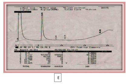
Figure (1): The Gas Chromatography pattern for Fatty acids standard. A. oleic acid, B. palmitic acid, C. Linoleic acid, D. Stearic acid, E. Thymoquinone
