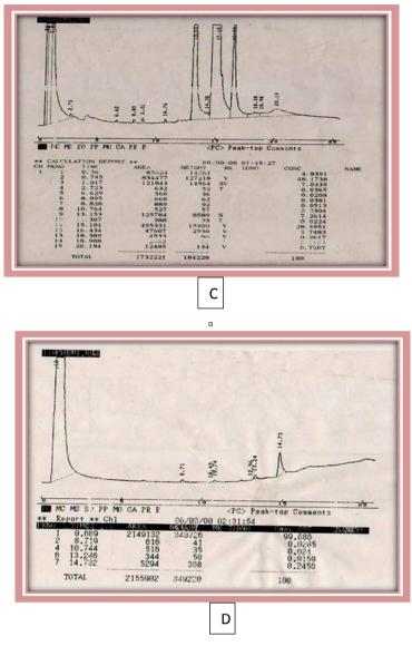
Figure (2): The Gas Chromatography for oil seeds extracted by different solvents. A. Aqueous extraction, B. Methanol extraction, C. Chloroform extraction, D. n- exane extraction.
