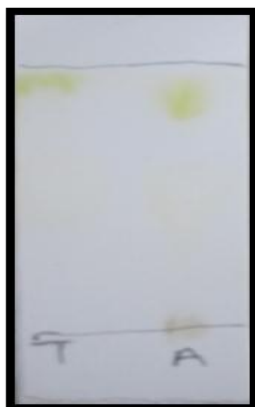
Fig. 2a Thin Layer Chromatogram of aqueous extract of N.sativa seeds in comparison with the standard Thymoquinone (T- Standard Thymoquinone and A- Crude Aqueous extract)
