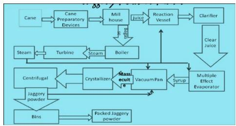
Fig. 5. showing Manufacturing of Jaggery Powder
