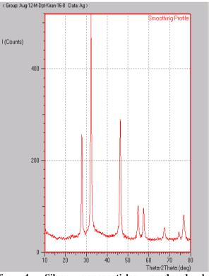
Fig. 4. Silver nanoparticles produced by *L.amylophilus* GV6 was analysed by X-ray diffraction for identifying its nature and size.
