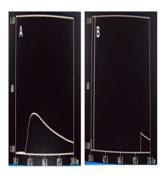
Fig. 2. Wavelength scan of silver nanoparticles produced by *L. amylophilus* GV6 by observing in a UV-visible spectrophotometer
