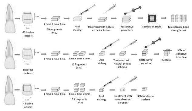
Figure 1. Schematic drawing of experimental design
