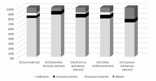
Figure 2. Graphical representation of percentages failure pattern of the different experimental groups.
