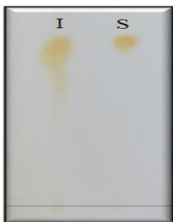
Fig. 1: TLC of profile of isolated (I; Rf 0.67) and standard (S; Rf 0.68) vasicine in ethyl acetate: methanol: ammonia (8:2:0.2 v/v).
