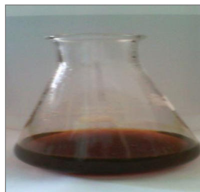
Fig. 3. Addition of flavonoid resulted in the colour change of AgNO 3 solution to dark brown
