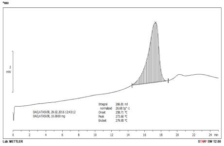
DSC thermogram of daclatasvirdihydrochloriderealed drug melting point at 273.60°C as in Fig.4
