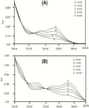
QU (375 nm) and CGA (328 nm) on a Systronics UV-Visible Double-beam spectrophotometer (model 2202).
