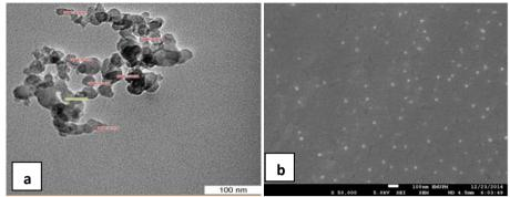
Figure 2: TEM micrograph showing homogenized, spherical shaped ciprofloxacin- cockle shells calcium carbonate (aragonite) nanoparticles (a), and FESEM micrographs showing dispersed and homogenized spherical shaped ciprofloxacin- cockle shells calcium carbonate (aragonite) nanoparticles (b)
