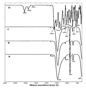
Figure 4: FT-IR spectra for micron-size cockle shells calcium carbonate aragonite powder (a), cockle shells calcium carbonate (aragonite) nanoparticles (b), ciprofloxacin-conjugated cockle shells calcium carbonate (aragonite) nanoparticles (c), and free ciprofloxacin (d) depicting the samples absorption or molecular interaction.
