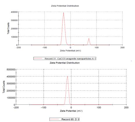
Figure: 3. Zeta potential distribution of cockle shells calcium carbonate (aragonite) nanoparticles (a), and ciprofloxacin- cockle shells calcium carbonate (aragonite) nanoparticles (b).
