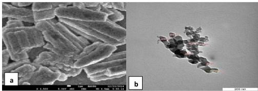
Figure 1: FESEM micrograph showing the pore structured of the micron-size cockle shells calcium carbonate powder (a), TEM micrographs showing synthesized, nanoscale, spherical-shaped cockle shells calcium carbonate (aragonite) nanoparticles (b)
