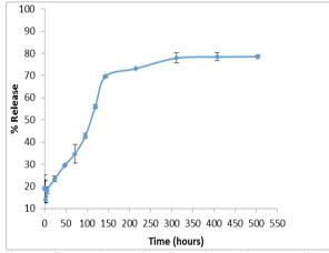
Figure 5: *In vitro* ciprofloxacin release profile of cockle shell calcium carbonate aragonite nanoparticles. Each bar represents mean  $\pm$  standard deviation (n=3) of three independent experiments.
