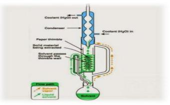
Fig. Soxhlet extractor
