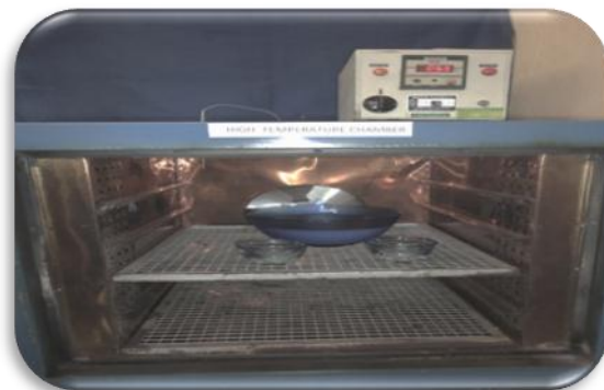
High temperature chamber 55 0 C (Accuracy \pm 1 0 C)
