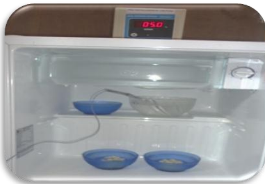
Low temperature chamber 5 0 C (Accuracy \pm 0.1 0 C)
