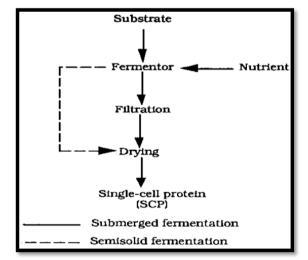
Figure 3: Flow chart of production of single cell protein by Fermentation process
