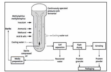
Figure 2: Flow chart of production of single cell protein from ICI UK.'Pruteen' plant
