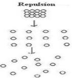
Water is drawn into the pores and particles repel each other due to the resulting electical force
