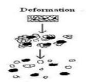
Particles swell to precompression size and break up the matrix
