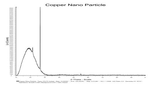
Fig. 3: XRD analysis of copper nanoparticles.
