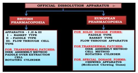
Common specification of various dissolution apparatus
