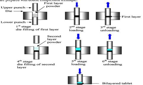
7<sup>th</sup> stage ejection Fig. 11: Steps Involved In Preparation of Bilayer Tablets.<sup>[13]</sup>
