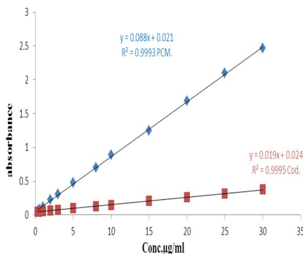
Fig. 2: Calibration curves of PCM and COD in mixture.
