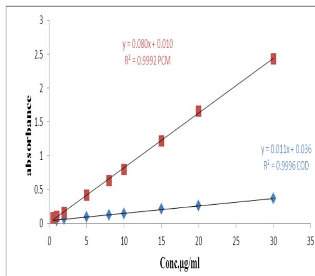
Fig. 3: Calibration curves of PCM and COD alone.
