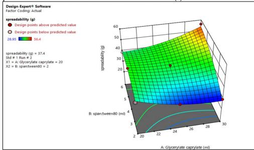
Fig. 3: Response surface depicting the effect of glycerylcaprylate and Span80:tween80 on spreadability.
