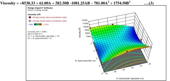
Fig. 4: Response surface depicting effect of glycerylcaprylate and Span80:tween80 on viscosity.
