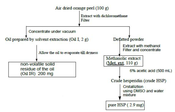
Figure 1: Flow chart for extraction and preparation of different fractions of orange peel: oil prepared by solvent extraction (OIL I), non-volatile solid residue of OIL I (OIL IR), methanolic extract (Met. ext.) and pure hesperidin (HSP).
