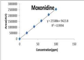
Figure 4: Calibration curve of Moxonidine.
