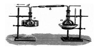
Combustion tube (b) contains in the centre a loose plug of platinized asbestos, which is kept in position by a
