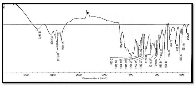
Figure 3: FTIR of Timolol Maleate with Croscarmellose Sodium.
