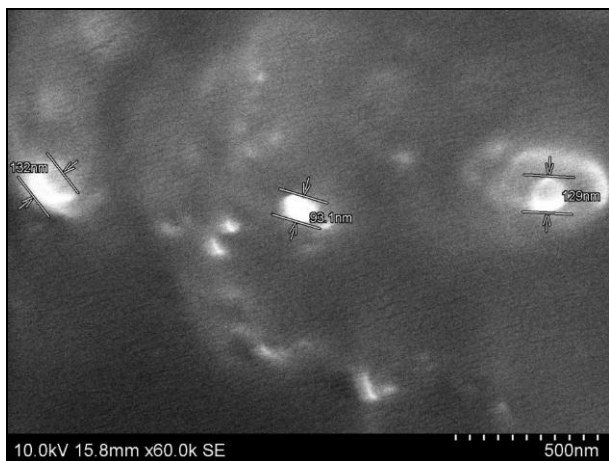
Figure 9: SEM image of optimized coated niosomal formulation at 60K magnification.
