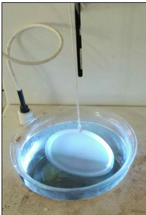
Figure 5: In vitro bioadhesion test assembly.
