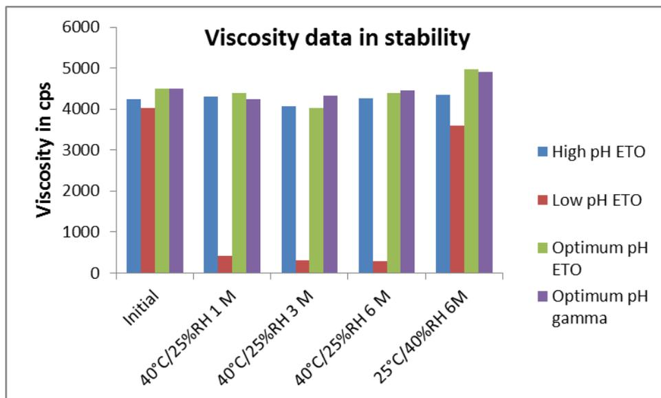
Fig 3: Viscosity data of pH range & container closure sterilization.
