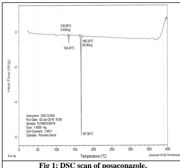
**Fig 1: DSC scan of posaconazole.**
