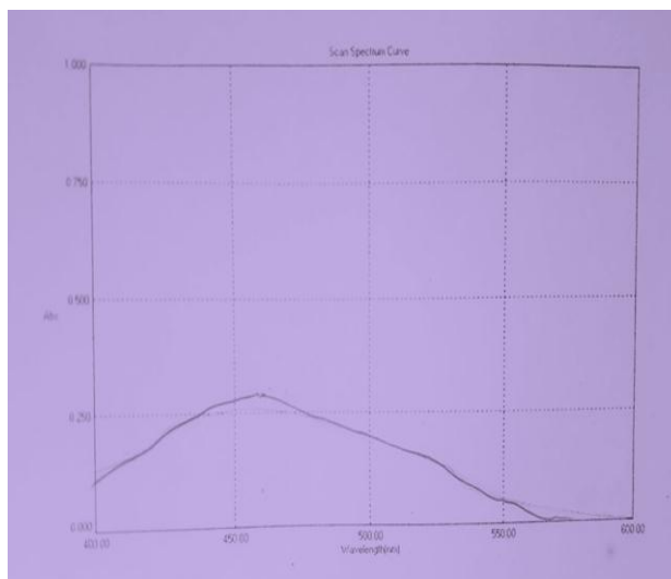
Figure 2: Absorption spectra of 20µg /ml of Vardenafil hydrochloride.
