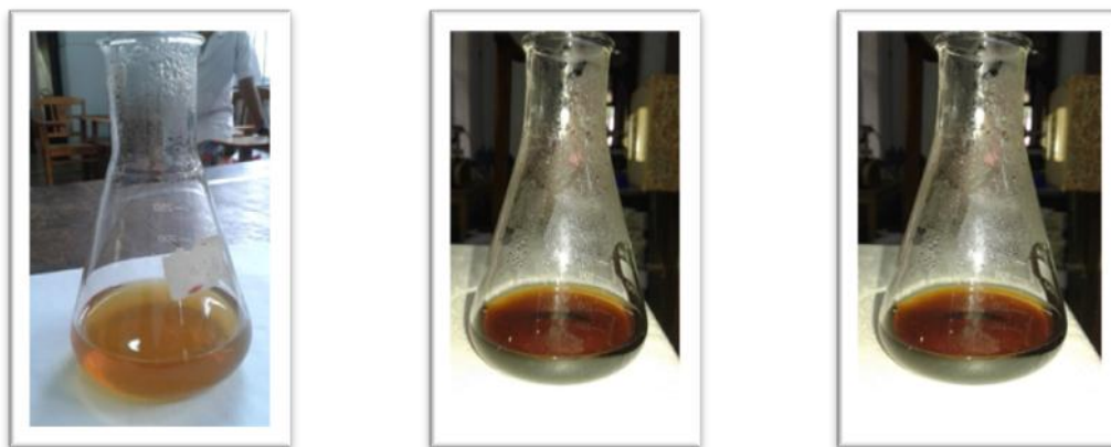
Fig 2: Synthesised silver nanoparticles indicated by yellow and yellowish brown colour from Plectranthus amboinicus , Azadirachta indica and Moringa oleifera .
