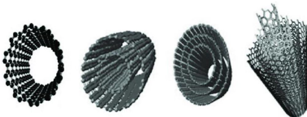
Fig. 3: Various types of carbon nanotubes: (A) Single-walled, (B) Double-walled, (C) Triple-walled, and (D) Multi-walled carbon nanotubes.
