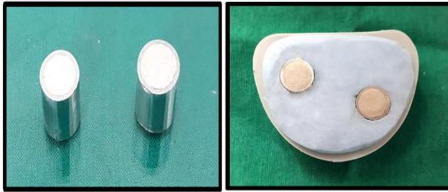
Figure 1: Steel pipe filled with plaster on glass slab for master die fabrication and mould made of polyvinyl siloxane material.
