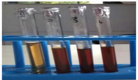
Different shades of copper nanoparticles during synthesis
