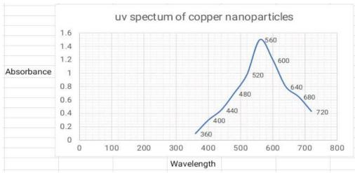
Fig. 5: UV Visible spectrum of copper nanoparticles.
