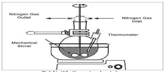
Fig.1: Liquid-liquid suspension polymerization.
