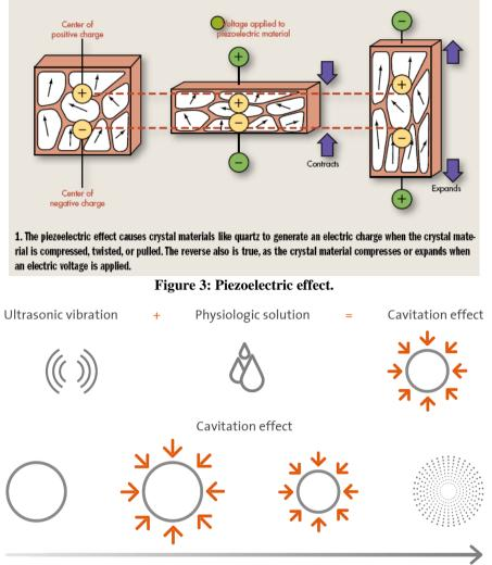
Increased static pressure Figure 4: Cavitation Effect.
