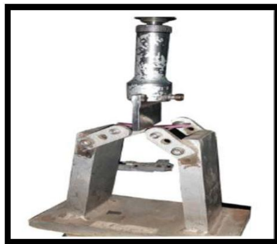
Fig 6: Flexural strength testing in Universal Testing Machine.
