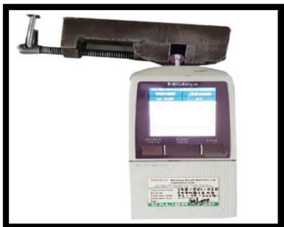
Fig 5: Surface roughness testing in Surface Profilometer.
