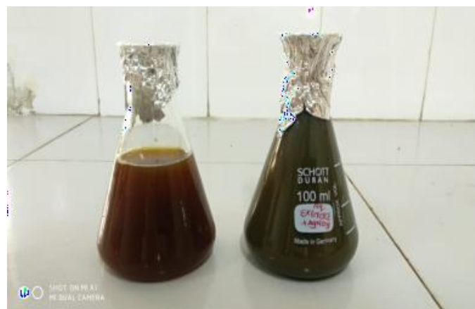
Fig. 2: Aqueous leaf extract of Cassia alata plant Before and After the Formation of AgNPs.
