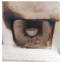
Fig. 1: Acid soluble ash value determination.
