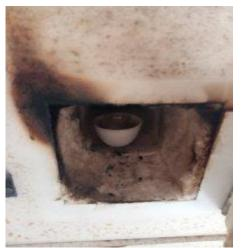
Fig. 2: Water soluble ash value determination.
