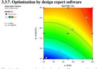
Fig.11: Countour plot showing the effect on carbopol and HPMC in *in vitro* drug release.
