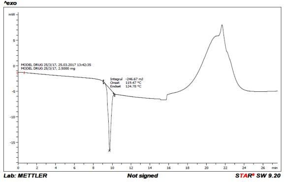
Figure 1: DSC Thermogram of Zidovudine.
