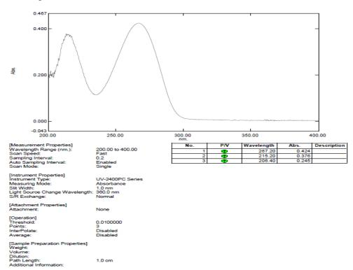
Figure 10: UV spectrum of Zidovudine in pH 4.5 acetate buffer.
