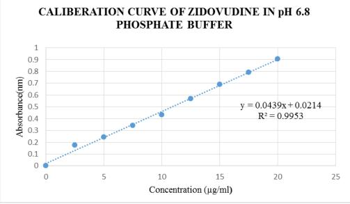
Figure 12: Calibration curve of Zidovudine in 6.8 phosphate buffer.
