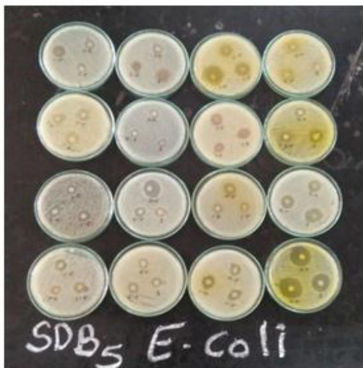
Figure 1: Effect of azo compounds of Resorcinol viz. 5a– 5h on the growth of E.Coli .
