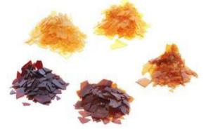
Fig.3 D. Shellac commercial resin marketed in the form of amber flakes
