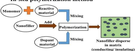
Figure No.6: In-situ polymerization method.
