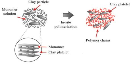
Figure No .14: Clay polymer nanocomposites.
