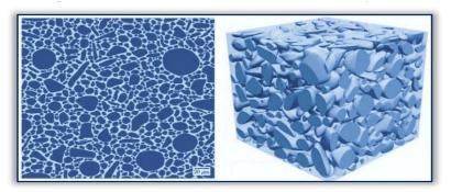
Figure No.3: Metal Matrix Nanocomposites.
